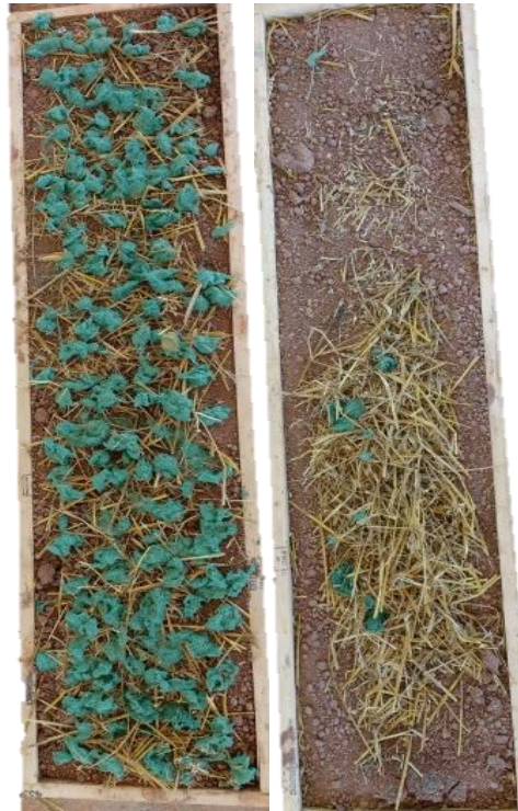
Figure 4: A before (left) and after (right) view of a soil test box with an application of hydraulic tackifier. This illustrates a “failure” with less than 50% of the straw remaining.
