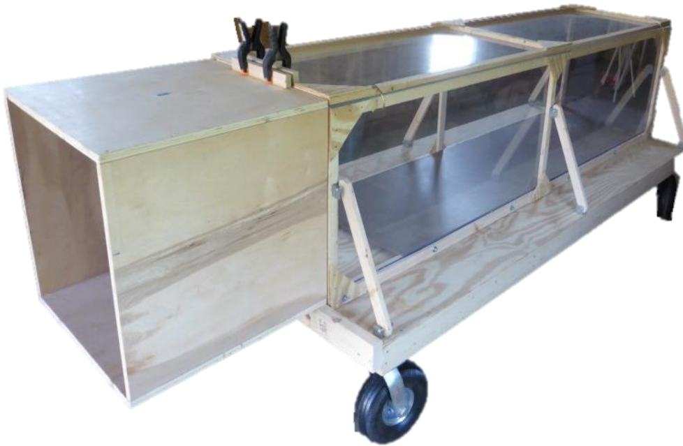
Figure A3: View of the wind tunnel with the laminar flow baffle section attached.
