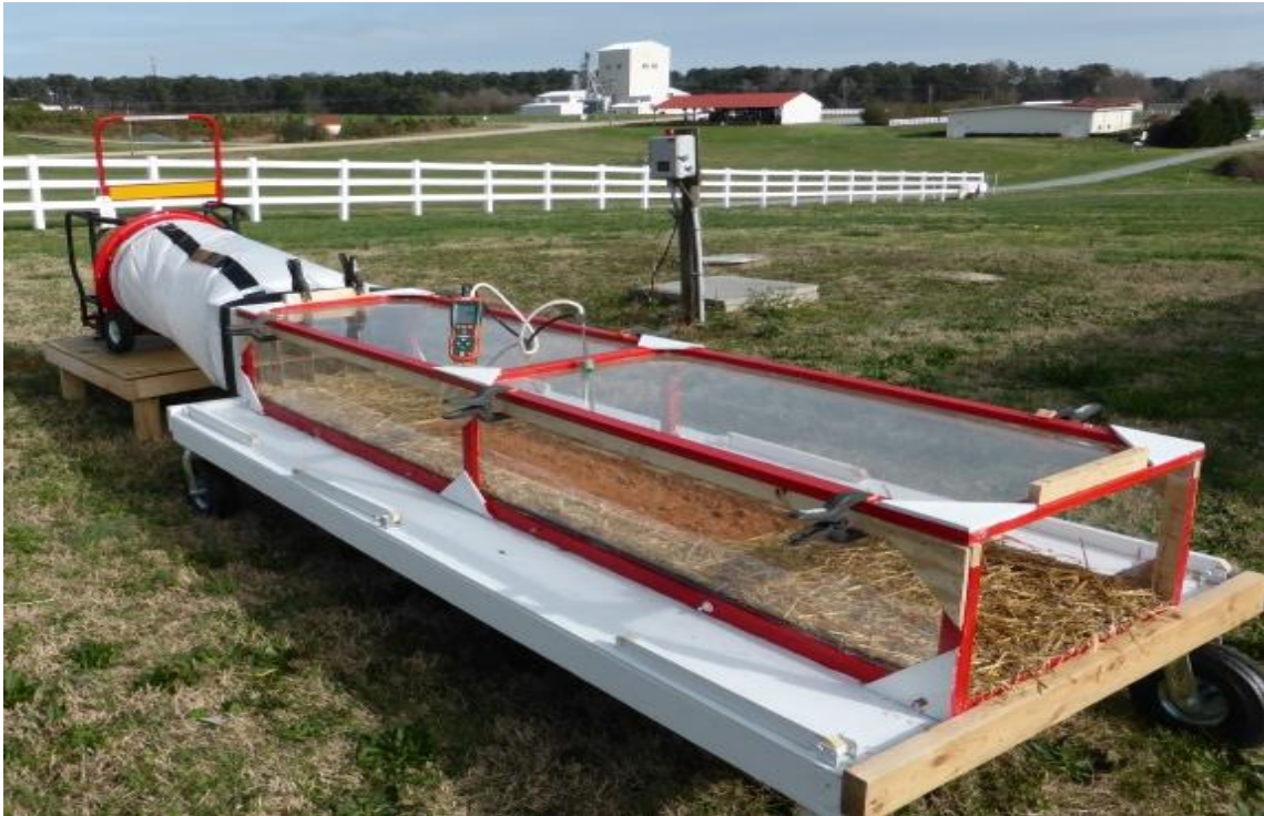
Figure 1: Fully operational wind tunnel with the fan properly attached and a bare soil box inside. The orange wind speed meter sits on top, exterior to the box, with only the probe on the inside.
