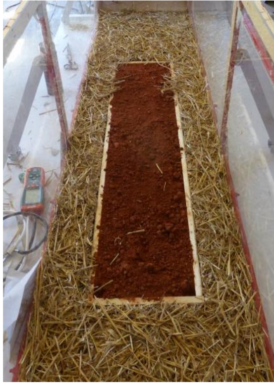
Figure 2: Test box filled with soil and installed in the wind tunnel. During testing, the box also has straw with or without tackifier applied to the soil.
