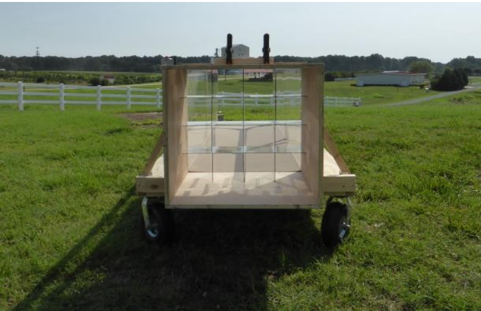
Figure A2: View of the wind tunnel through the section connecting the fan to the tunnel, with laminar flow baffles.
